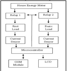
Fig. 7 Block Diagram of Limiting Device
